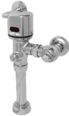
The Hydrotek H-8000C Sensor Flush Valve is the AC powered variant of the 8000C series flush valves. Dependable and versatile, the vandal resistant brass construction is available in many configurations and is field adjustable for left and right rough-in as well as convertible from/to urinal or closet allowing the most flexibility in the installation and maintenance in each unit.
