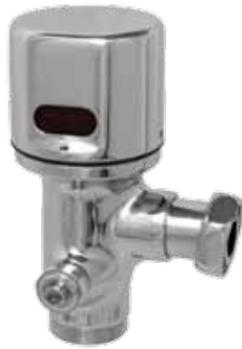
The Hydrotek HB8RFKC is a battery operated, retrofit sensor flush valve that is the most dependable and versatile electronic flushing system in the industry today. Installation is quick and easy as it utilizes your existing Sloan, Delany, Zurn, or Toto stop valve, vacuum breaker and flush tube.
