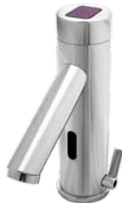
The 7000SLEM Series faucet is a solar sensor faucet that provides a vandal resistant, no touch lavatory solution with hot/cold mixing that promotes better hygiene and energy savings. These faucets use ambient light to function and utilizes a battery back-up.
