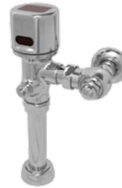
The Hydrotek H-8000SLE Solar Flush Valve is built upon the same reliable and versatile electronic flushing system as the 8000C series sensor flush valves, but powered by a solar cell that will generate more energy savings on top of the excellent water savings the 8000 series flush valves provide. Rated for 650,000 flush cycles, this valve can last up to 10 years before needing the battery back-up replaced.
